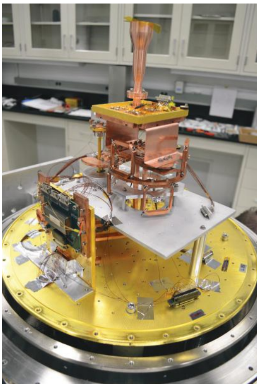
Model 104 hosting optical testing of detectors at John Hopkins University. Image: David Larson, CLASS collaboration
